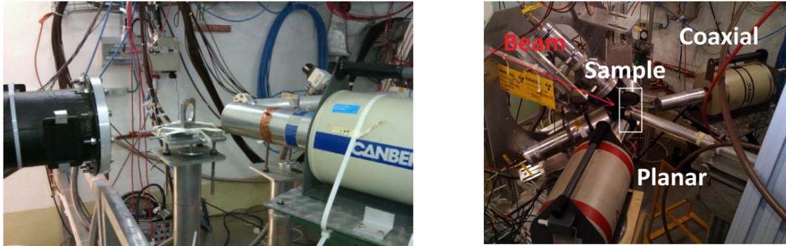
Figure 1: Several HPGe detectors tested a n_TOF with different commercial electronics [1].
