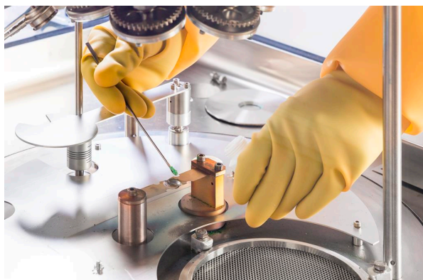
Fig. 1: Loading the tantalum filament of the ^{238}\text{U} -evaporator with ^{238}\text{UF}_4 powder for the preparation of a ^{238}\text{UF}_4 deposit by physical vapour deposition.
