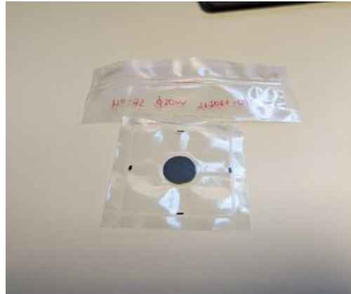
Figure 24: Picture of the 95 Mo pellet sealed under vacuum in a thin plastic bag.
