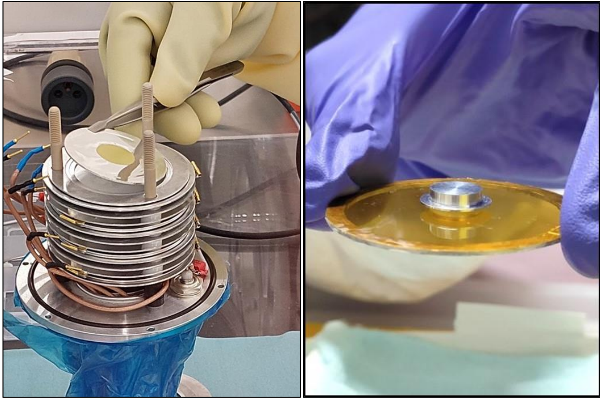
Figure 1 Left: picture of the mounting process of one \text{PuO}_2 sample in the fission chamber. Right: picture of the actual capsule containing the thick sample during its mounting between two aluminum rings with kapton and mylar foils (the top mylar ring does not appear in this picture).
