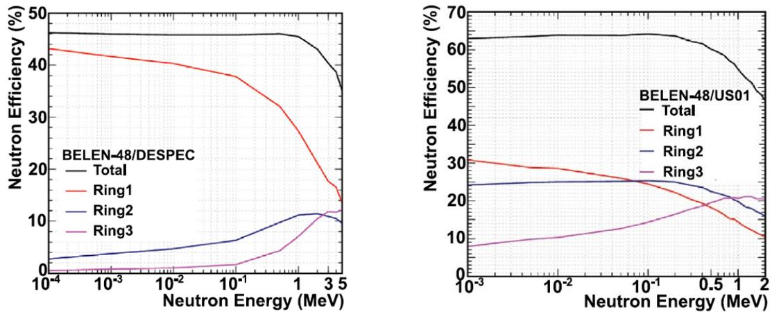
Figure 12. Neutron detection efficiency for the original BELEN-48 detector (left) and for the optimized for low  $Q_{\beta n}$  windows (right)
