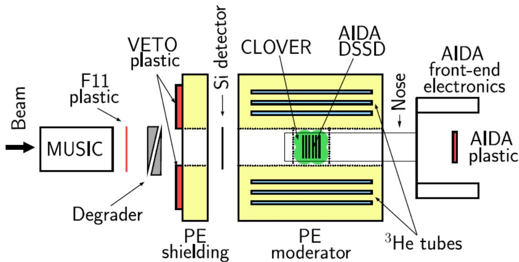
Figure 5. Arrangement of elements in the experimental setup (drawing not to scale)
