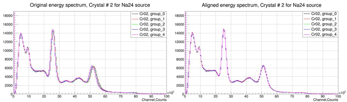
Fig. 1 Example of the alignment procedure, to correct the gain shifts, that occur during the data taking. On the left panel, the raw spectra from crystal#2 are presented. On the right panel the same data after alignment is presented. This procedure has been already performed for all detectors and for all measured cases including the calibration sources.
