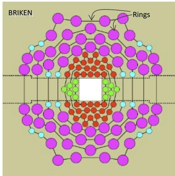
Figure 1. BRIKEN detector geometry.
