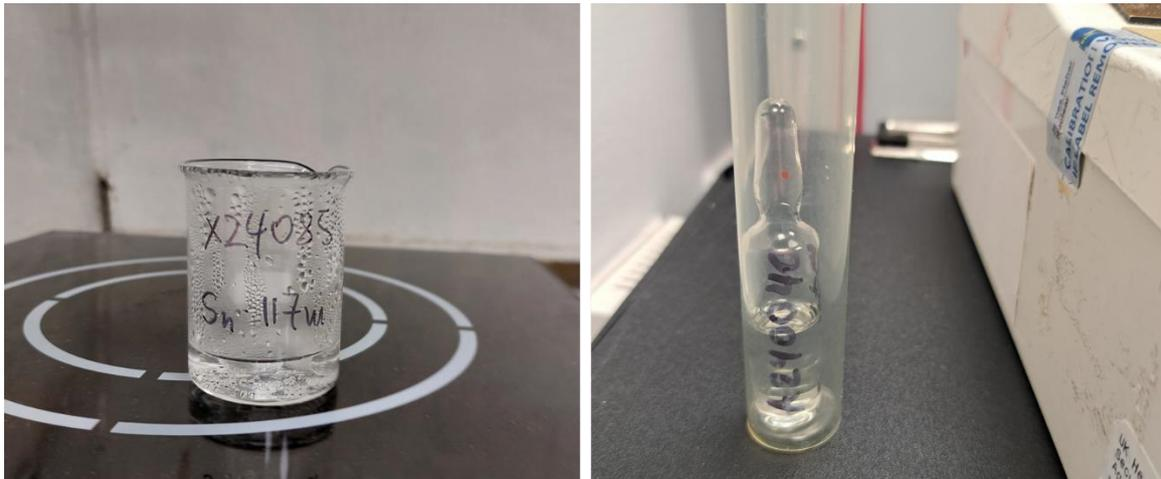
Figure 3: Photographs from the radiochemistry suite at NPL. The left picture shows the tin foil dissolving in 10 mL of 6M hydrochloric acid on a warming plate. The right picture shows the 5 mL ISO glass ampoule.
