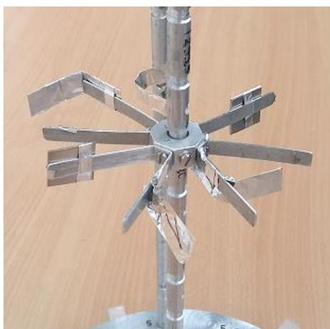
Figure 32. View of the metal foils fixed to the aluminum holder.
